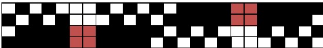
Bedford cord weave, 10 threads cord with 2 waded ends
